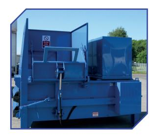
The KHD 3000 is a high performance compactor. A reliable and proven machine that can be used to compact commercial or industrial waste and even recyclable materials such as cardboard. The KHD comes as standard with high safety features including low 24v operating controls, dual safety monitoring circuits and E-stops at control positions.
