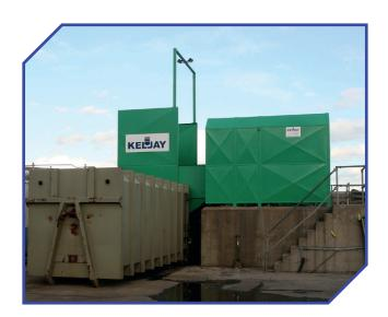
The KHD 6000 is our largest static waste compactor, a colossal machine suited to very large waste through puts or bulkier materials. This machine is ideal for seaports, large waste facilities and other large scale operations. The 6000 comes as standard with high safety features including low 24v operating controls, dual safety monitoring circuits and E- stops at control positions.
