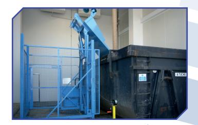
The HD mobile is a great versatile tipping system most commonly utilised when tipping waste bins or containers into open top skips. However, with Keljay's bespoke manufacturing capabilities our mobile tipping systems can be tailored to your requirements to enable you to tip with containers and to heights of your choice.
