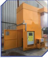
The high lift tipper with anti-scatter hood is designed to tip waste material such as flour into large waste containers. The anti-scatter hood encompasses the whole of the tipping area significantly reducing the amount of excess dust and particles generated by fine waste product that can escape and soil the surrounding working area during the tipping process
