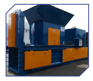
The Auto 800 Baler is our largest baler in our semi automatic range. This machine is extremley powerful, capable of producing cardboard bales of 700kg and more. The A800 is also complete with large loading aperture for speed and ease of loading. This Baler is designed for maximising lorry and shipping container payloads. This machine has the option for either 4 or 5 wire tie.
