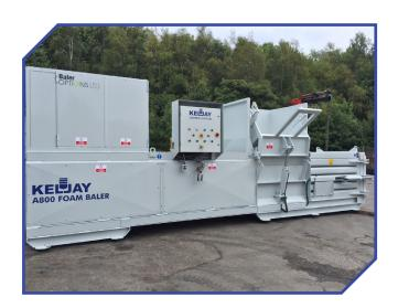
TThe A800F is a specialist semi autmatic baler, purpose built for the baling of foam and other difficult materials. This machine enables bales to be tied by up to 8 ties, 4 horizontally and 4 vertically over the bale. Producing bales of up to 550kg in weight this baler is perfect for maximising transport pay loads.
